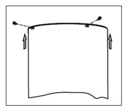
**7)** Slide the upper chimney section upwards and then use the self tapping screws (3 pcs) to secure it to the hanging plate.
