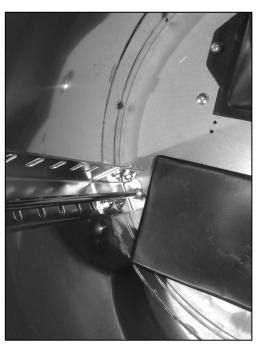
**5)** Use the 10 mm x M4 nuts and bolts with metal washers (6 pcs) to secure the main body of the hood to the angle bars.
