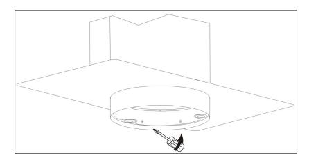
$\circ\,$  Use a screwdriver to retighten the 6 fixing screws that hold the light board in place.
