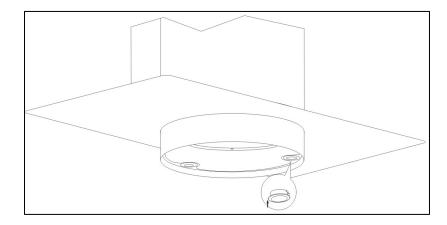
Push the light back into the exposed hole in the hood and reconnect the light wiring point (see page 23 for a line drawing that shows how to reconnect the light wiring point).
