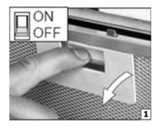
1) Remove the grease filter.
