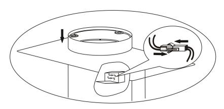
Carefully locate the glass canopy over the main body of the hood.
