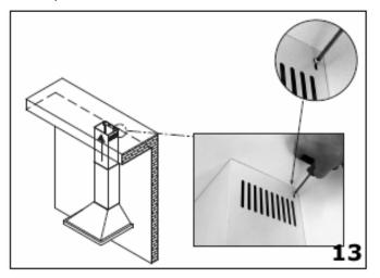
Slide chimney section D inside of chimney section C. Then secure the upper bracket to the wall, using the same method as you have just used to secure the lower bracket.
