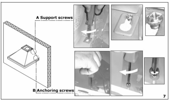
**7)** Fully tighten the support screws **(A)** and then screw the anchoring screws **(B)** through the relevant holes in the cooker hood. Fully tighten the anchoring screws fully into the wall.
