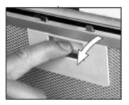
1) Remove the metal grease filters.
