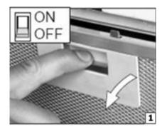
1) Remove the grease filters.
