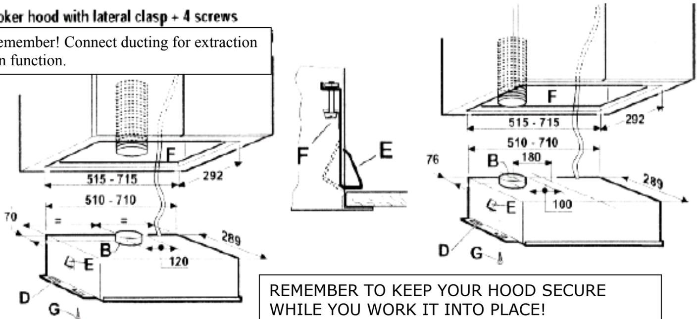
**7) Finally, fix the cooker hood to the cabinet with the wood screws supplied ('G' in figure above on right).**
