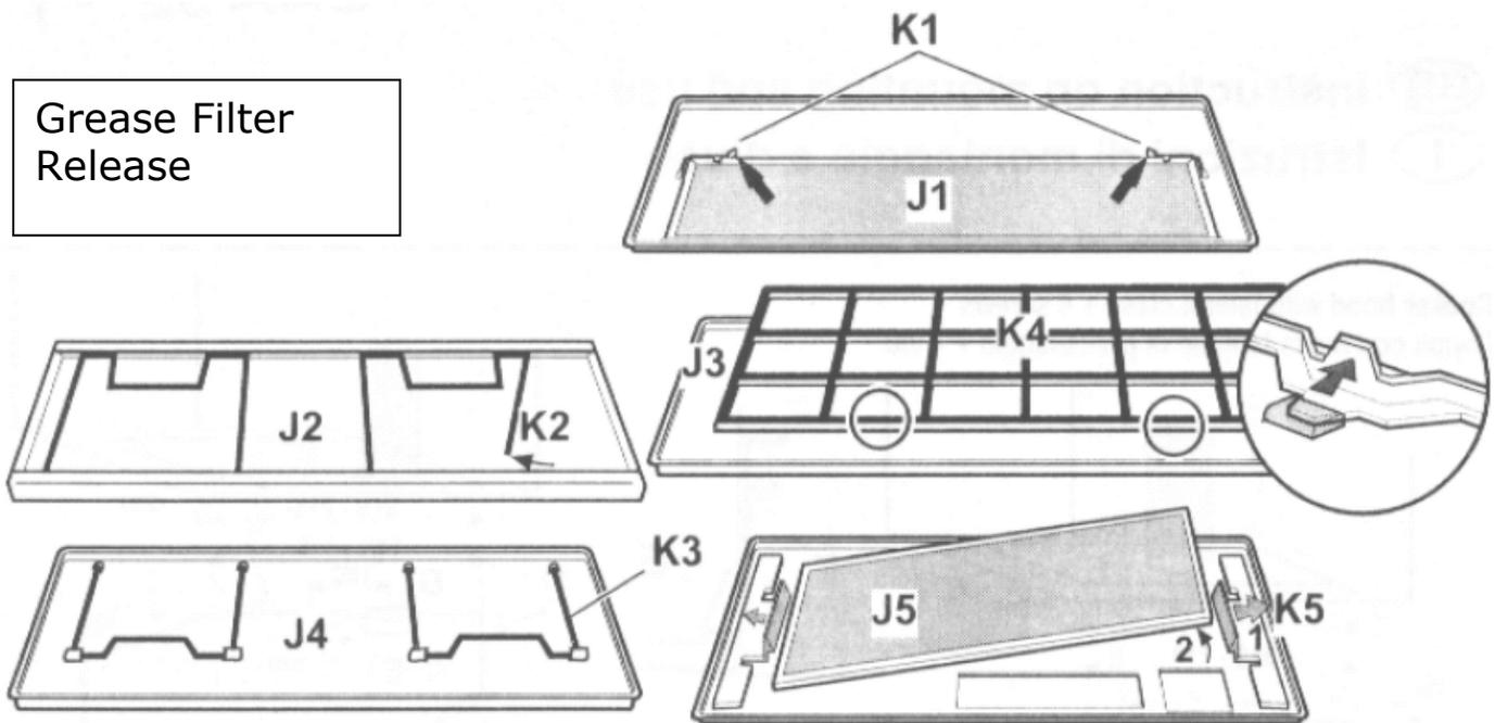
**First remove the grease filter grille by turning in the two lugs on the underside of the grille.**
