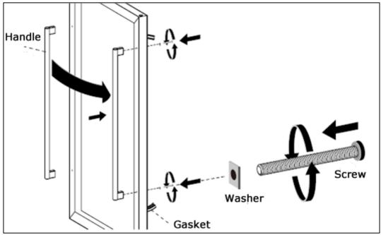
4) Install the 2 decorative screws in the holes on the left hand side of the outer door by following the instructions for removing the decorative screws in reverse (step 1).
