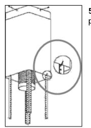
**5)** Fix the upper chimney section to the hanging plate, using the 4 x self tapping screws.
