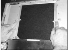
4) After inserting the front edge of the carbon filter into the slot on the cooker hood. Lower the back edge of the carbon filter, until it clicks into place at the rear of the rectangular hole. Raise the two fixing bars, until they are horizontal over the carbon filter.
