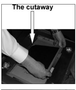
3) Insert the carbon filter in the rectangular hole, fitting it over the motor.
