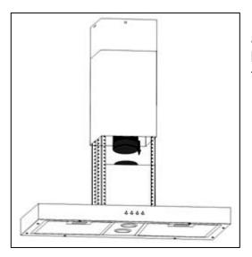
**8)** If you are going to be using the hood in extraction mode, you should fix the ducting hose to the spigot.
