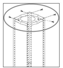
**2)** Fix the angle bars to the hanging plate, using the 8 x M4 nuts and bolts with metal washers.
