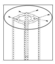
2) Fix the angle bars to the hanging plate, using the 8 x M4 nuts and bolts with metal washers.
