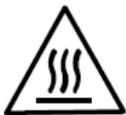
This label, positioned on the rear of your dryer, indicates that the surface is hot when in use so avoid touching it.
