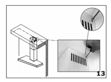
**13)** Lift chimney section **D** up to the ceiling and secure it to the fixing bracket using the screws provided.
