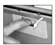
1) Remove the metal grease filters.
