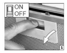
1) Remove the grease filters.
