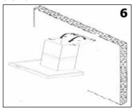
**6)** Hang the hood onto the support screws.
