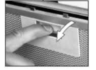
**1)** Remove the metal grease filter.
