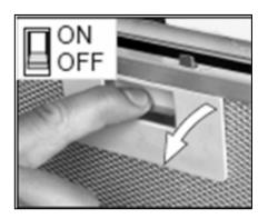
$\circ~$  Refit the grease filter.
