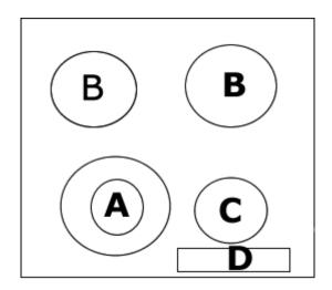
A = 3.30 kW wok burner B = 1.75 kW semi-rapid burner C = 1.00 kW auxiliary burner D = Control panel
