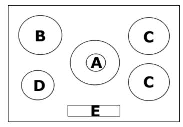
A = 3.80 kW wok burner B = 3.00 kW rapid burner C = 1.75 kW semi-rapid burner D = 1.00 kW auxiliary burner E = Control panel
