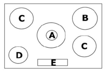
**A** = 3.80 kW triple crown (wok) burner
