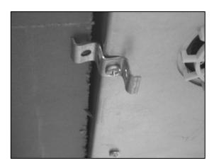
base or the sides on the hob that you can fix the four brackets to. There are three holes in each one of the brackets.
