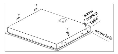
Carefully turn the hob back over and then gently lower it into the aperture hole that you have cut out.
