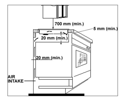
o **IMPORTANT:** You must observe the ventilation requirements shown in the drawing above. In particular the 20 mm gap underneath the hob and the 5 mm gap underneath the front edge of the worktop.
