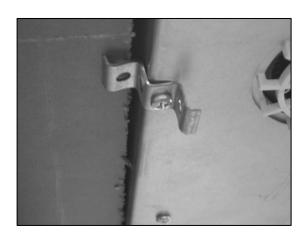
You should place the bracket on the underneath of the hob, in a position that is appropriate for the aperture that you have cut out. Using the screws provided, fix the bracket to the hob. These screws MUST be securely tightened.
