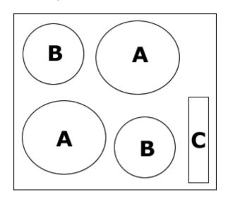
A = 1.80 kW radiant zones B = 1.20 kW radiant zones
