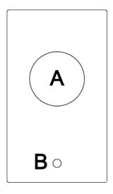
A = 3.80 kW triple crown (wok) burner
