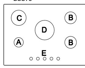
A = 1.00 kW auxiliary burner
