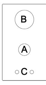
**A** = 1.00 kW auxiliary burner
