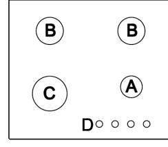
A = 1.00 kW auxiliary burnerB = 1.75 kW semi-rapid burner
