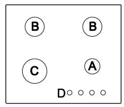
A = 1.00 kW auxiliary burner
