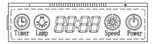
o When you initially connect the cooker hood to the electricity supply, the backlight will turn on and the hood will enter standby mode. If no buttons are pressed the backlight will turn off again after 30 seconds.
