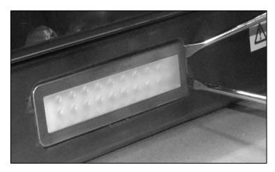
o Once the light unit has been released from the fixture, gently pull out the light unit.
