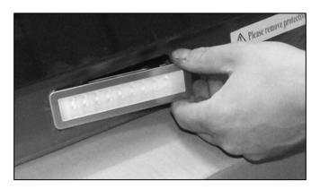
There are wires connected to the back of the light unit. Once you have pulled out the light unit and wires a short distance, you can disconnect the wires by pulling them out of the connectors.
