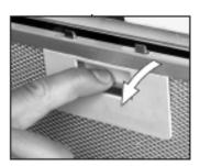
1) Remove the metal grease filter.
