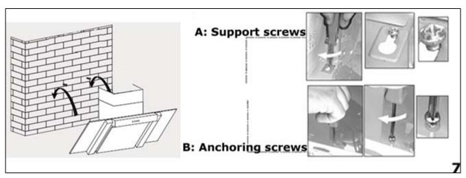
**7)** Fully tighten the support screws **(A)** and then screw the anchoring screws **(B)** through the relevant holes in the cooker hood. Tighten the anchoring screws fully into the wall.
