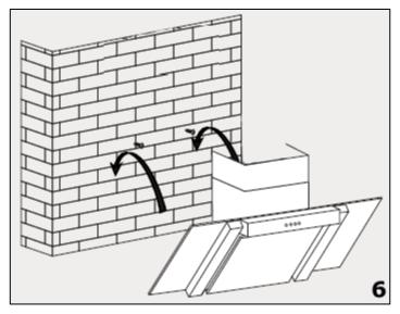
**6)** Hang the hood onto the support screws.
