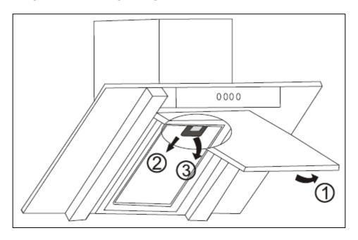
Lift up the cover that sits over the grease filter (as shown in the line drawing above).
