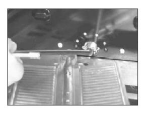
Free the burners from their fixing screws.
