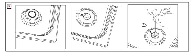
Unscrew the injector and replace it with the required injector for the new gas supply according to the table below.
