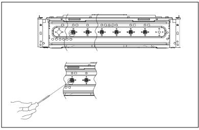
Locate the adjusting screws for the grill and oven burners. These will be positioned to the left hand side of the grill and oven thermostat taps.
