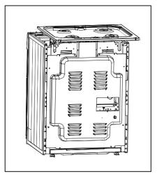
When all the screws have been removed, slide the hob from the back to the front and lift it off the support brackets which hold the hob down at the front of the cooker.
