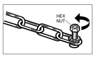
To fix the security chains to their anchor brackets: Loosen the hex nut at the unattached end of the safety chain, until it is flush with the screw end. Do not remove it completely.
