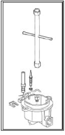
Unscrew the injector and replace it with the stipulated injector for the new gas supply (see table below).
