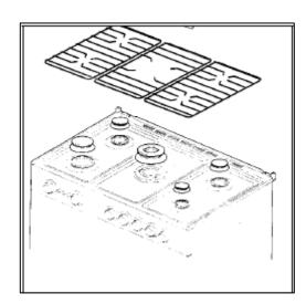
Remove the pan-stands, burners and flame spreaders.
