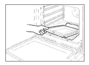
Remove the burner base from the bottom of the oven.
