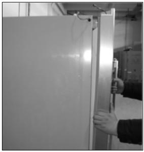
o Whilst still supporting the door, slowly lift it upwards to disengage it from the lower hinge. Once the door has been lifted clear of the lower hinge, pull it away from the main chassis of the appliance.
