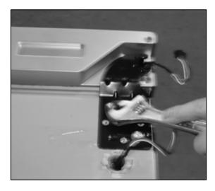
o Undo the three bolts that hold the upper hinge in place.
