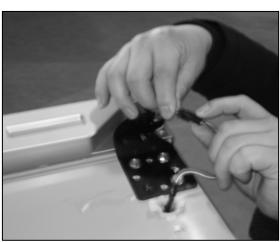
o Disconnect the electrical connection point that sits underneath the hinge cover.
