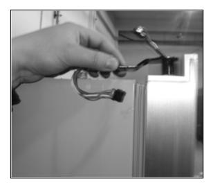
o **IMPORTANT:** One person should support the door before attempting this next step. Lift up the front of the hinge and remove it from the appliance.
