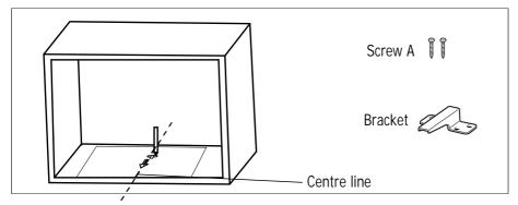
3. Remove the bottom cabinet template and fix the bracket with screw A.
