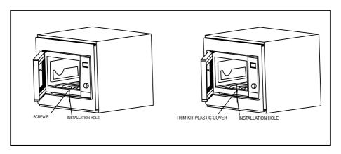
2. Open the door; fix the oven to the cabinet with SCREW B at the INSTALLATION HOLE of TRIM KIT. Then fix the TRIM-KIT PLASTIC COVER to the INSTALLATION HOLE.
